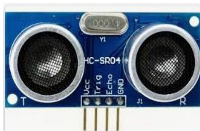
Gambar 2. Sensor Ultrasonik HC-SR04
